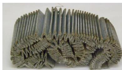
Fig. 2: The mixed bed demineralizer inlet filter after being cut
