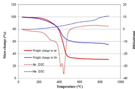
Fig. 9: Result of TG-DSC measurement when the commercial equipment specimen is heated in a He stream and an air stream
