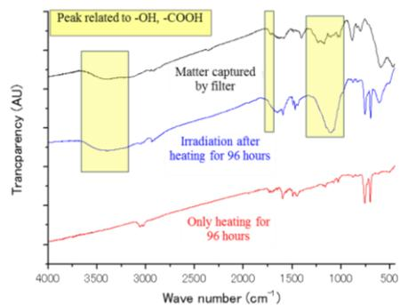
Fig. 5: FT-IR spectra of the mock specimen and the commercial equipment specimen
