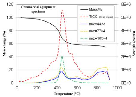
Fig. 8: Result of TG/MS measurement when the commercial equipment specimen is heated in a He stream
