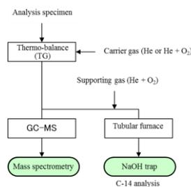
Fig. 7: Experiment flow for checking the thermal decomposition behavior of hardly soluble particulate C-14
