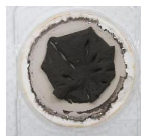
Fig. 3: Particulate components captured on the 0.45  $\mu\text{m}$  MF
