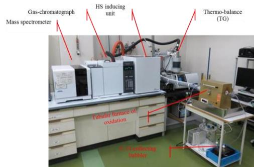
Fig. 6: Experiment apparatus for checking the thermal decomposition behavior of hardly soluble particulate C-14
