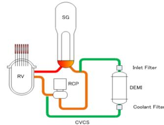
Fig. 1: Schematic diagram of the primary cooling system and the chemical and volume control system of the PWR
